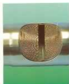
The rare-metal catalytic converter is designed to last longer than ceramic types.
