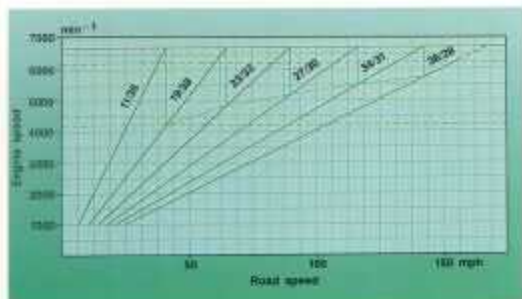
Transmission designer's chart: The 6-speed transmission's gear ratios were selected to allow exceptional flexibility - freeway speeds are attained with a single 1st-2nd upshift.
