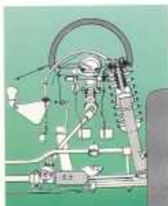
Segmented steering column is designed to deflect the column in a frontal collision.
