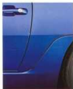
Aerodynamic side skirts with integral stone guards are blended fluidly into 968 design.
