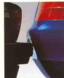
The new soft bumpers are designed to withstand impacts of up to 3 mph without damage.
