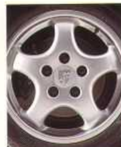
Light-alloy wheels help meet the chassis engineer's "handling" goal of low unsprung weight.
