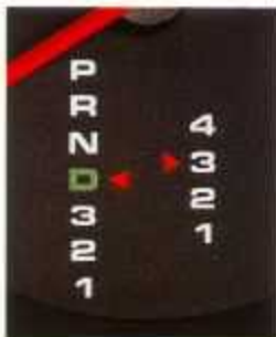
The mode and gear currently engaged are displayed on tach-mounted LEDs.
