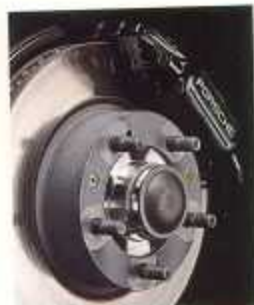
Massive 4-piston fixed-caliper brakes are lifted directly from racing.
