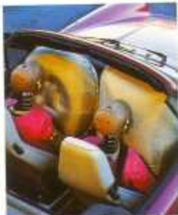
The 968, like all 1992 Porsches, provides air bag restraint systems for driver and passenger.
